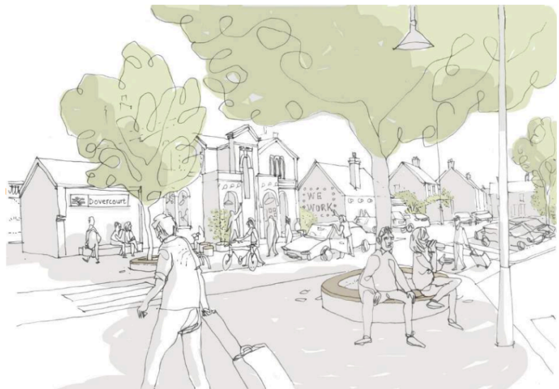
Figure 4.24: Sketch of station plaza proposals, including footway build-outs, formalised parking and drop-off, tree planting and seating
